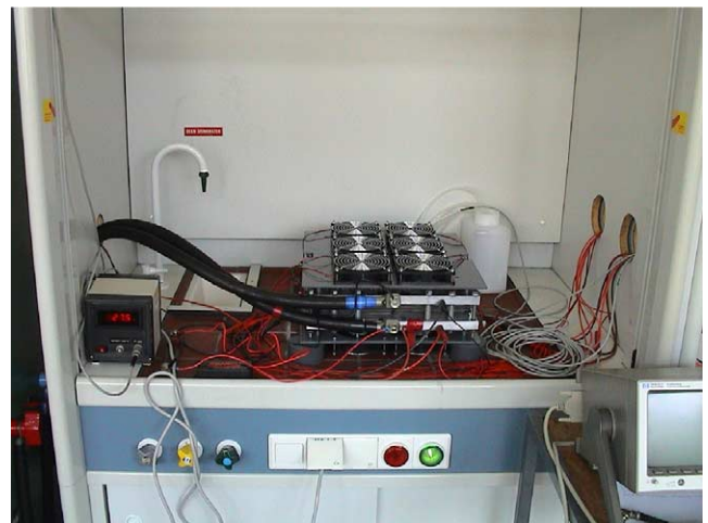
Fig. 4. Photograph of bipolar lead–acid battery under PALC testing.
